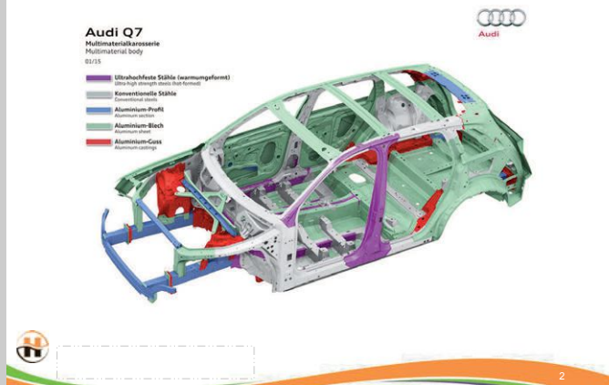
Figure 2 | Many vehicle manufacturers are incorporating more high-strength steel and aluminum into their vehicle frames. Gray and purple are conventional and ultra-high-strength steel, respectively. Blue, green and red are aluminum sections, sheets and cast parts, respectively. Black is carbon fiber reinforced plastic and yellow is magnesium. (Figure courtesy of Houghton International.)
