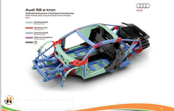
Figure 2 | Many vehicle manufacturers are incorporating more high-strength steel and aluminum into their vehicle frames. Gray and purple are conventional and ultra-high-strength steel, respectively. Blue, green and red are aluminum sections, sheets and cast parts, respectively. Black is carbon fiber reinforced plastic and yellow is magnesium. (Figure courtesy of Houghton International.)
