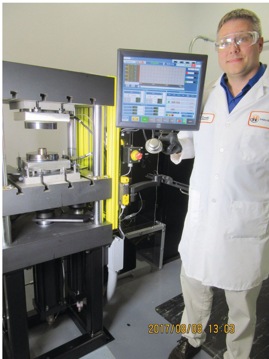
Figure 4 | Houghton chemist Scott Lay inspects an advanced high-strength steel cup made with the state-of-the-art Valley Forge Labs 40-ton stamping press that the company uses to evaluate new technologies. (Figure courtesy of Houghton International.)
